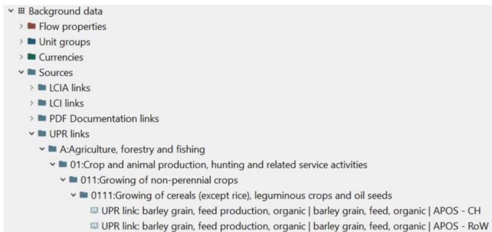
Figure 7: Example of new ecoinvent v.3.3 sources in the navigation pane of openLCA 1.5
