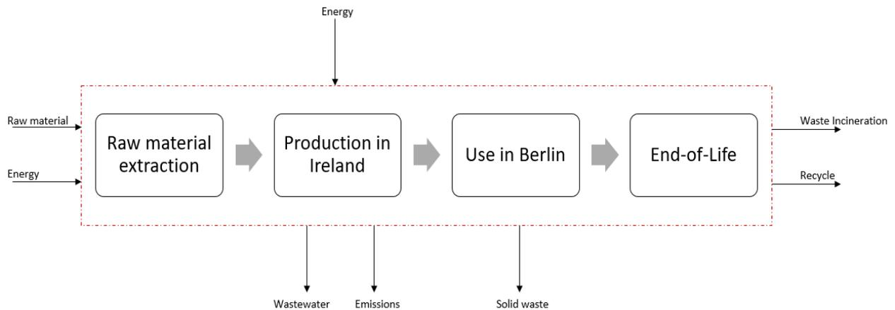
Figure 2 Process flow scheme for the Oral-B dental floss.
